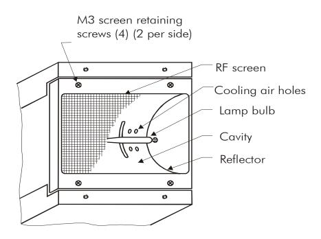
Figure 19. Reflector Assembly (I300M)
